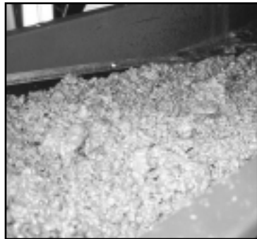
Flo-Line Primer removing large drilled cuttings at 10 mesh
