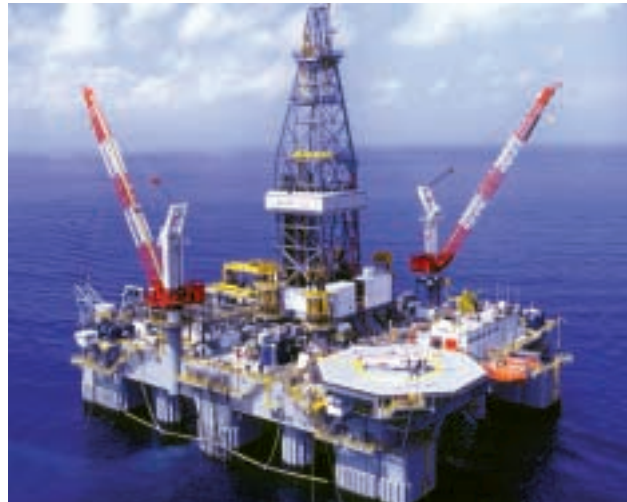
The Marine 700, a semi-submersible capable of operating in 5,000 ft. of water, offers one of the most environmentally-sensitive solids control systems available.
